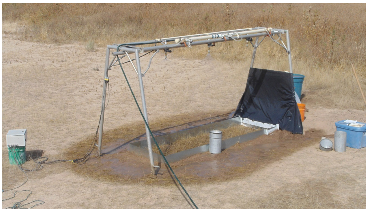
Figure 2. Modified Miller rainfall simulator (1987) used in plot experiments.
