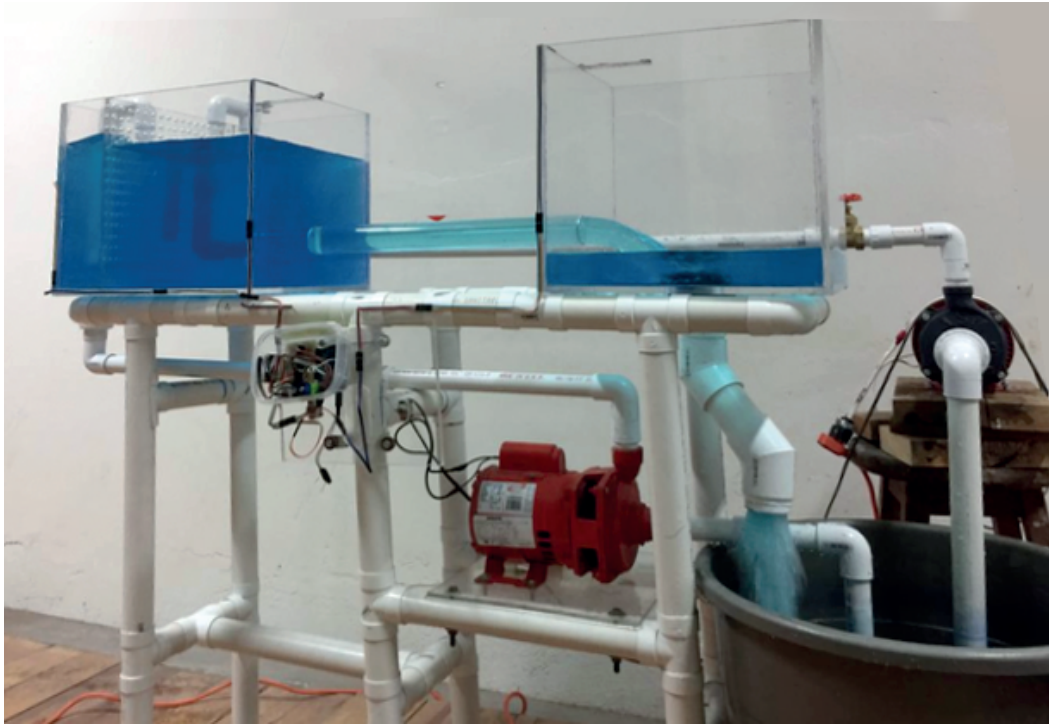
Figure 7. Operation of the hydraulic model as an orifice with free discharge.
