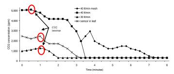
Figure 4. CO<sub>2</sub> concentration measured under different flows with mesh.
