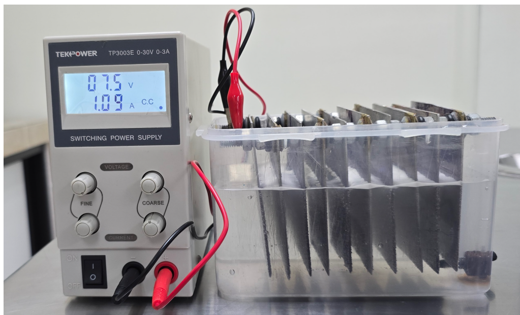
Figure 1. Scheme of the electrocoagulation unit used in the experiment.
