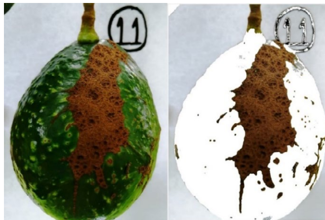
Figure 7. Original image of an avocado fruit (left) and an image where green pixels were changed to white (right) and counted to estimate the percentage of green pixels in an image. The percentage of green color found in this image was 42.92 %.
