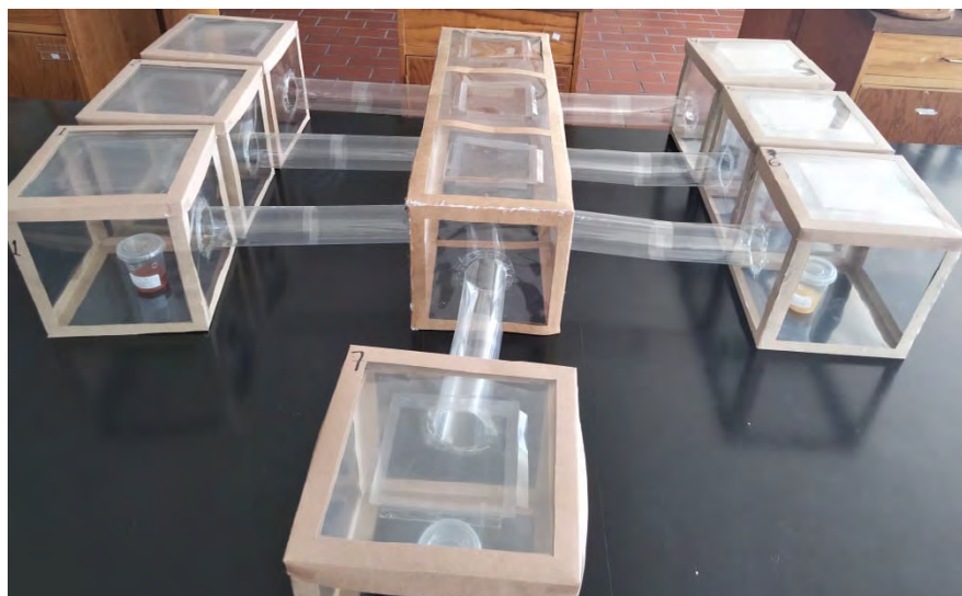
Figure 2. Trap Design I for evaluating attractants for the black fig fly ( Silba adipata McAlpine) under laboratory conditions.
