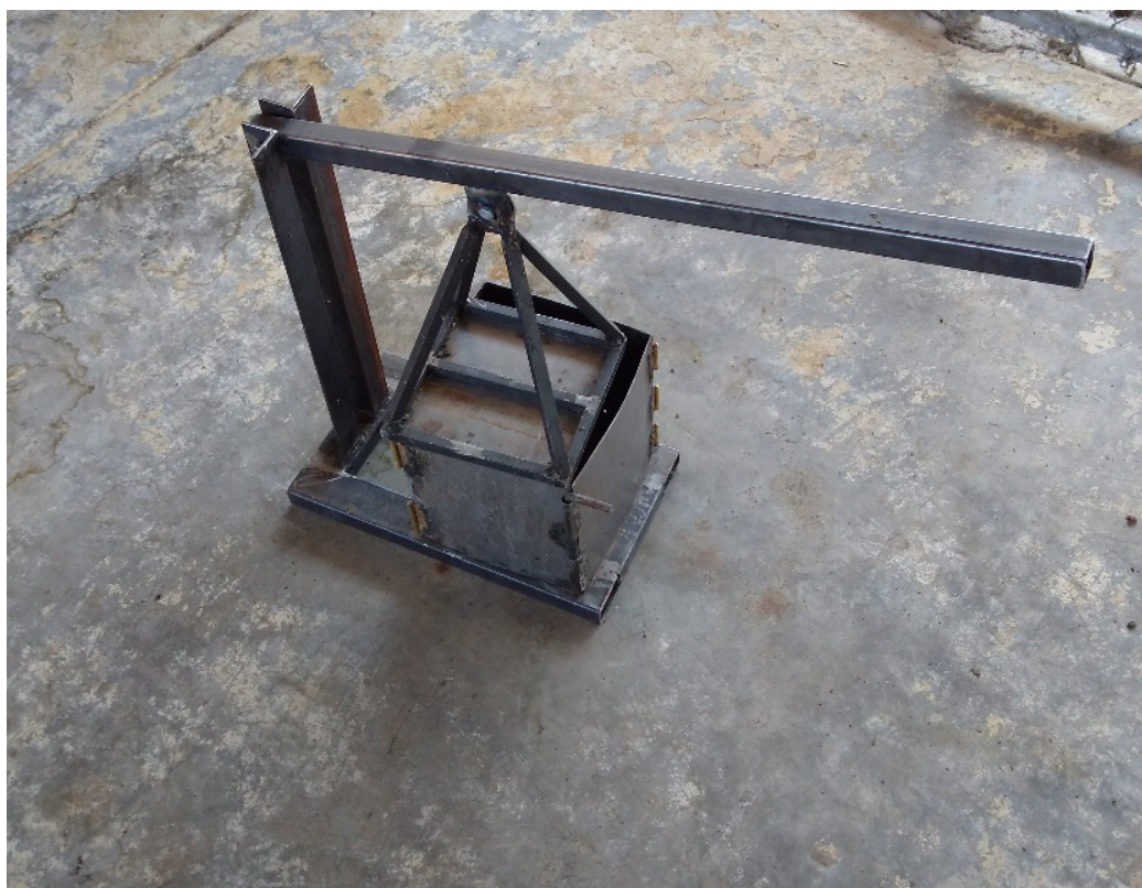
Figure 3. Metallic mold used for the handmade manufacture of the RNB. La Estrella, Pénjamo, Guanajuato.
